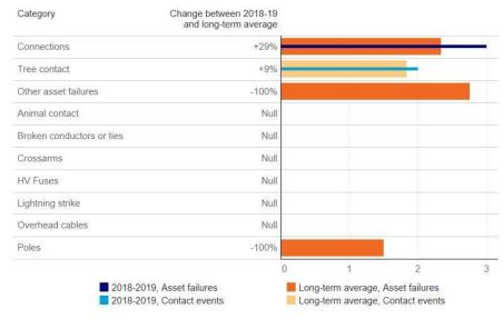
Figure 42 Incidents on the CitiPower network resulting in ground fires
