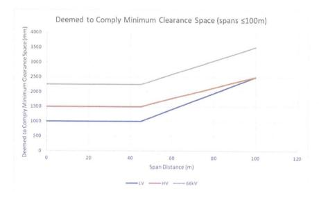
2. Allowance for sag and sway method: Specify a constant *applicable distance* to which an allowance for sag and sway must be added to calculate the minimum clearance space, MCS = AD+sag+sway.
