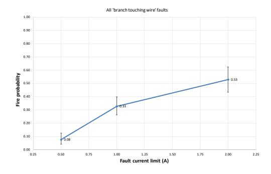
Fire risk can be cut by more than 90% if the supply is interrupted when the fault current reaches 0.5 amps
