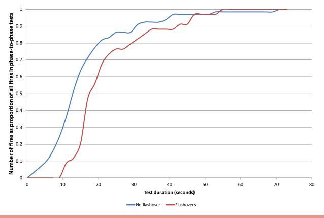
Fast (<5s) fault detection and response would cut fire risk by 90% (response time for 'branch touching wire' faults could be up to four times longer than shown for the same result).
