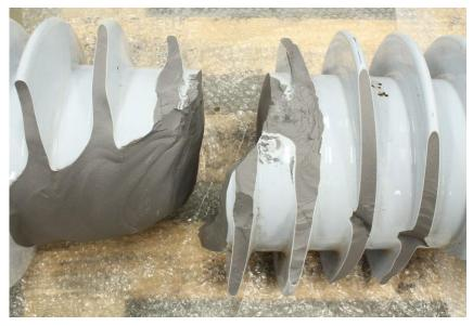
Figure 2: Close-up view of the two main sections of the failed insulator
