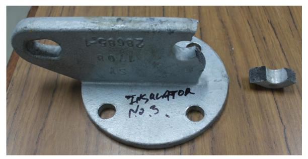
Figure 8: Image of a failed bracket after the mechanical failing load test
