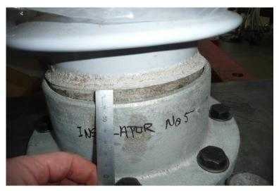
Figure 7: Insulator 5 after completion of mechanical failing load (MFL) test.
