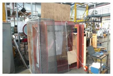
Figure 6: Image of the insulator loading frame for the insulator mechanical failing load test, in accordance with AS/NZS 2947.1
