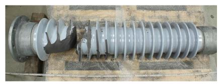
Figure 1: Overall view of the two main sections of the failed insulator
