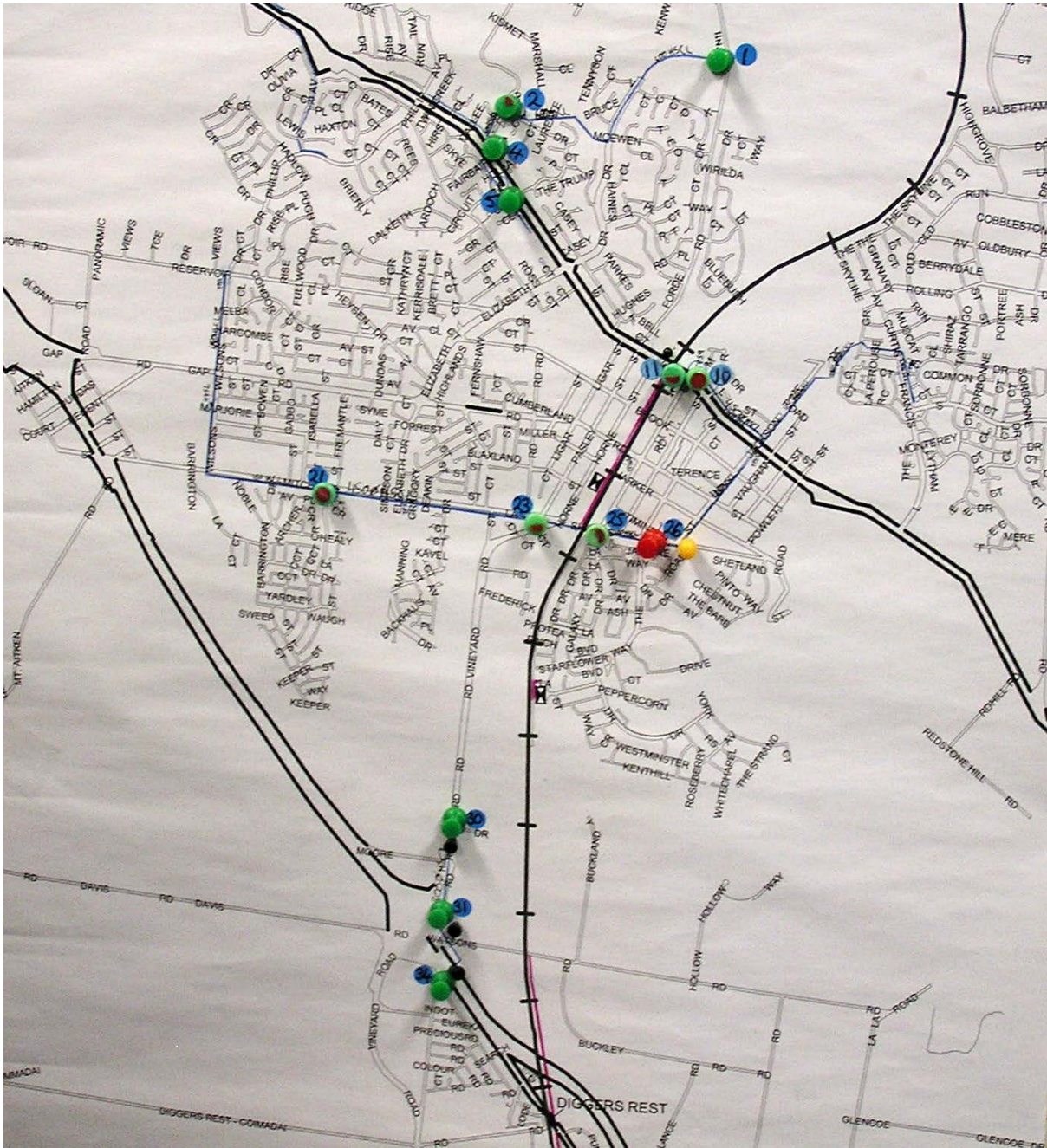
A typical map showing drainage bonds, electrolysis feeders, test points, ICCP systems and underground structures as used during combined area testing.
