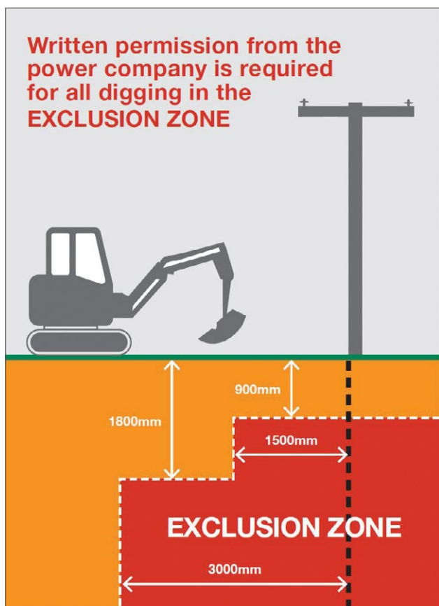
Figure 29: Excavation near poles
