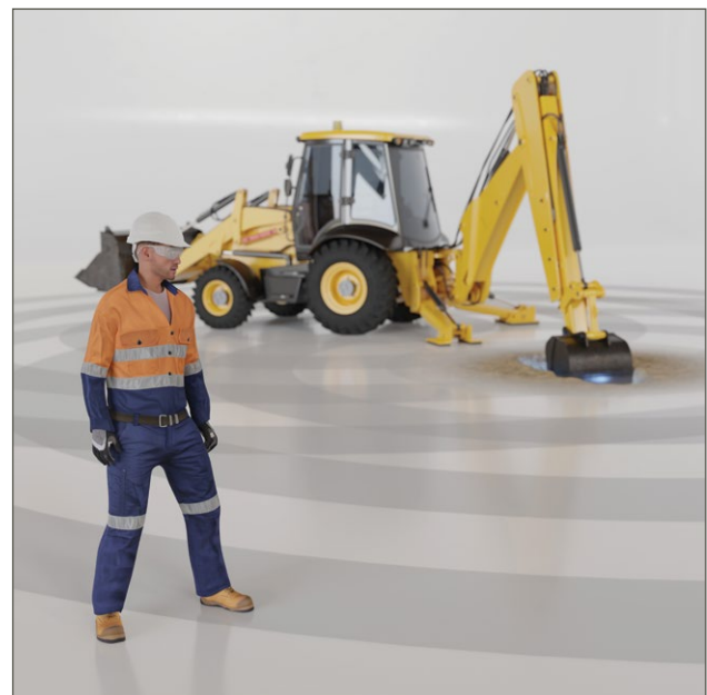
Figure 31: Step potential risk if an underground electrical cable is hit by the bucket
