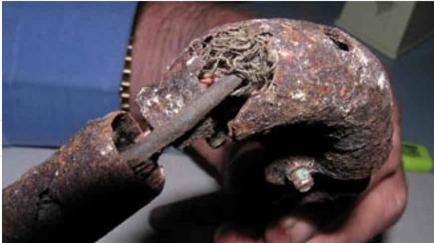
A section of deteriorated and "live" split conduit (See this page).
